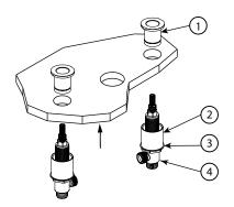
Remove top fastening nut and washer (1) from the lavatory valve. (NOTE A: All lever handle sets are supplied with one right-hand valve and one left-hand valve. Install valve with blue dot o the cold side [Round handle sets are supplied with two hot valves that turn in the same direction]). Insert valve from below through hole in lavatory or countertop.
