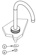
Insert spout base nipple into center hole in lavatory or counter top. Install stainless washer (5) nut (6) on spout nipple and tighten
