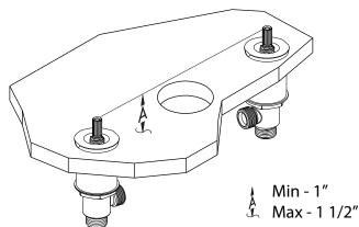
Set valve to proper rough-in height "A", by adjusting bottom - fastening nut. Secure valve by tightening top fastening nut. Repeat procedure for the second lavatory valve.
